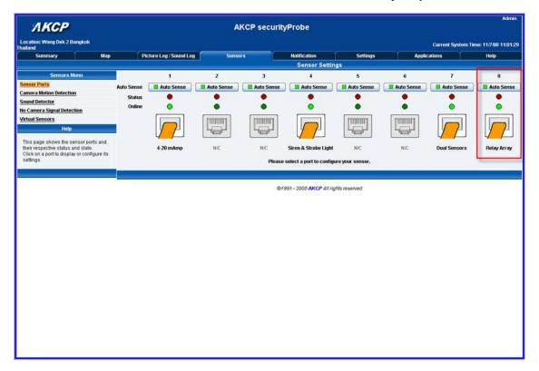
After clicking on the Relay Array we can see all our relay tabs and setting for each relay in the array, including our advanced settings.
